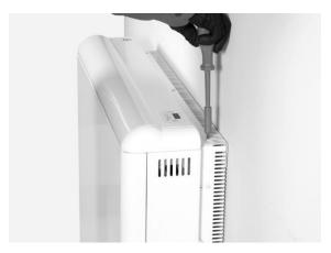
ECOHHR MUST NOT BE HUNG ON THE SCREWS; these are used only to prevent the device from overturning and not to support it. If there is any doubt concerning the wall strength, consult the corresponding construction specialist. The appliances are heavy; it is the installer responsibility the correct installation and wall support of these devices to prevent them from overturning.
