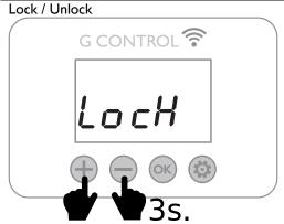
During any operation mode, it is possible to lock the keyboard by holding and simultaneously for 3 seconds. When the keyboard is locked, the message **Lock** will be displayed.
