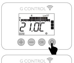
It is possible to modify the general setting. During any operation mode, press & release  $\bigcirc$ , the display shows the flashing temperature symbol  $\bigcirc$  and the RF symbol  $\bigcirc$  RF.
