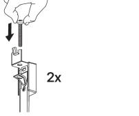
Place the screw in the bracket. (Don't screw it in fully.)
