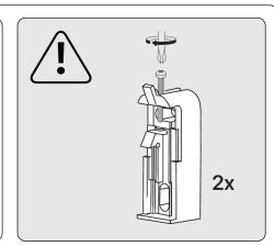
Screw the fixing screws into the brackets to secure the radiator.
