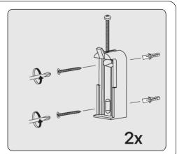
Attach the brackets to the wall, using the wall plugs and screws.
