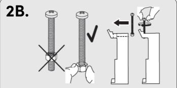
Twist the nut onto the tip of the screw and place into the
