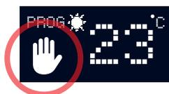
You can easily override, **until next program period**, the current program temperature by altering the temperature (you can set 10 to 30 °C) with
